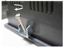
Please install the metal retaining bracket on the side of VX 760T, with the metal clip hooking the front cap and the top of the screw pushing against the inside of the control box.
