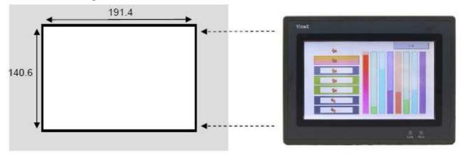
Please place the HMI with its back facing the opening side of the machine.
